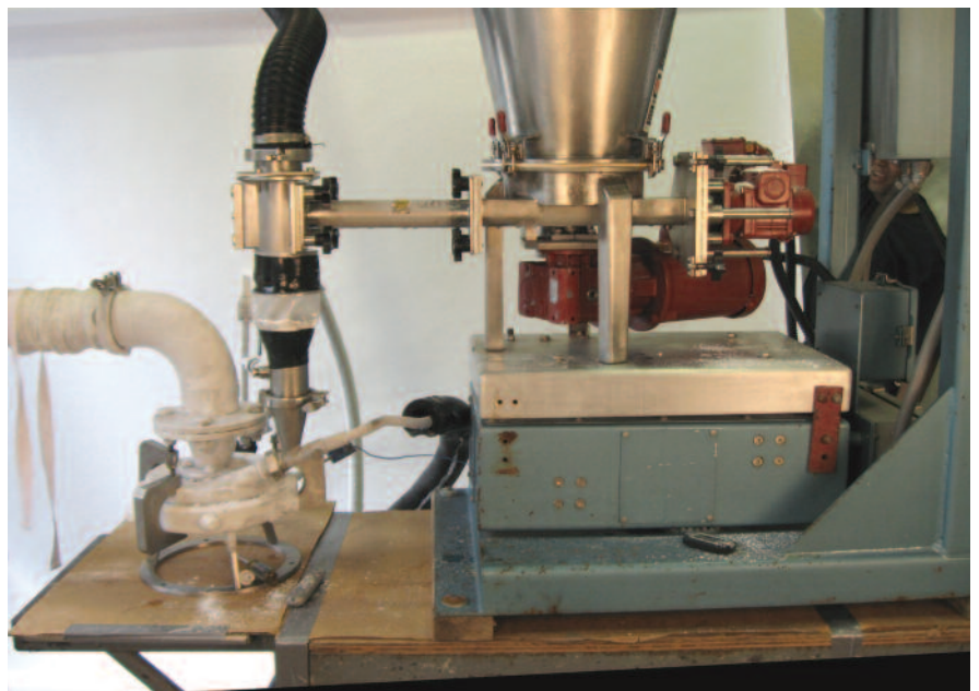
The cryogenic jet-milling system uniformly mills a heat-sensitive powder to a mean particle size range of 8 to 12 microns.
