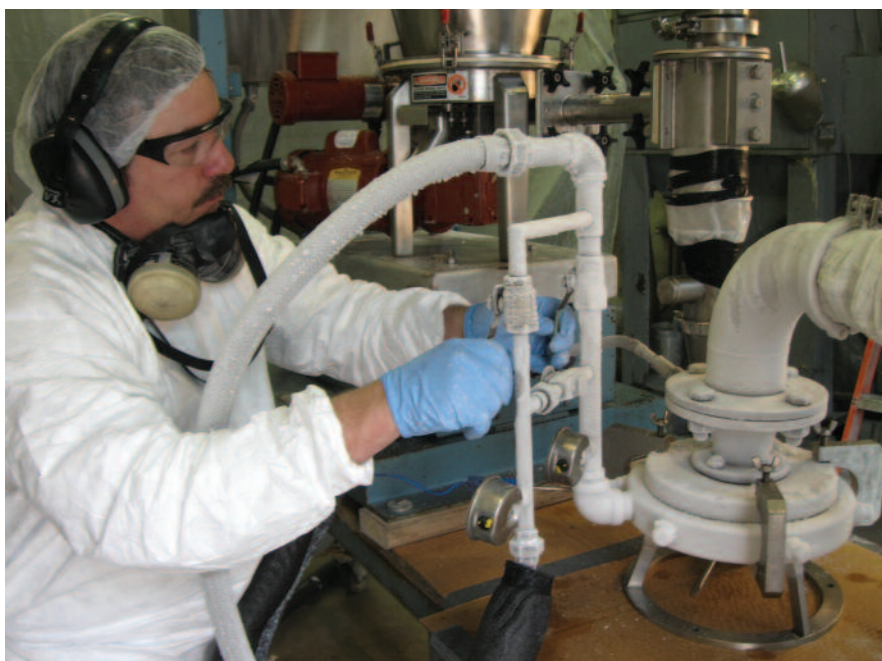
An operator adjusts the jet-milling system's operating parameters to ensure a quality finished product with no material loss.
